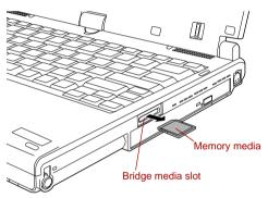
Figure 3-7 Removing memory media
